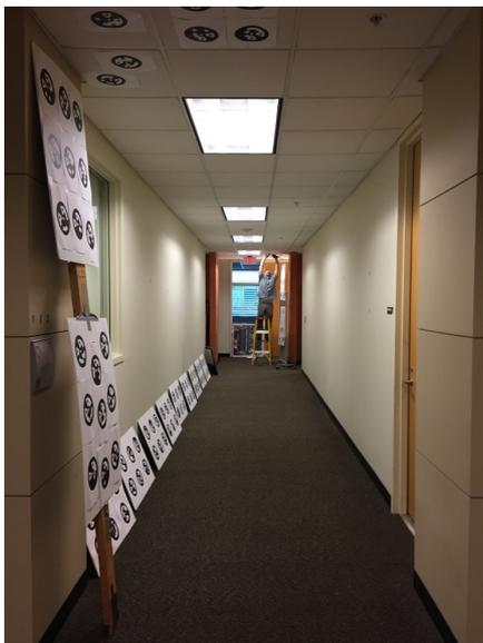
Figure 3. Indoor localization testing, using the mounted fiducials for the Intersense IS-1500 tracking system.
